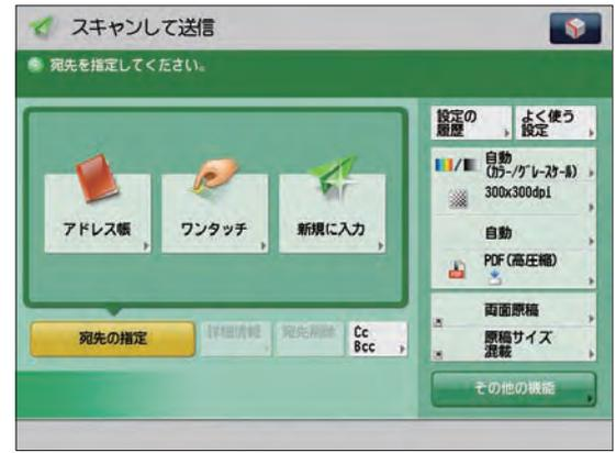
From the Scan to Send Screen, you can specify sending destinations, the resolution, file format, and other relevant settings to send your electronic document. Plus, you can register frequently used settings as shortcuts, which you can access from the lower right area. This further enhances your workflow efficiency.
