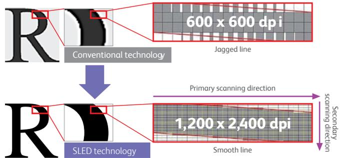
Gradation control in secondary scanning direction enables smoother reproduction of black lines and character outlines. This feature is especially effective on the lines in low angles. The result is smoother, sharper image reproduction.
